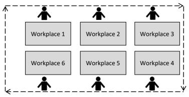
This is what a conveyor with a workplaces rotation looks like in its simplest form. There is a difference from the classic conveyor. There, people are attached to the workplace, and the product moves along the conveyor, but people do not move. In a conveyor with a rotation of workplaces, workers are not profiled for a single operation, they are not "married" to it. They know how to do every operation of the entire process. They move together with the product in diverse workplaces.
