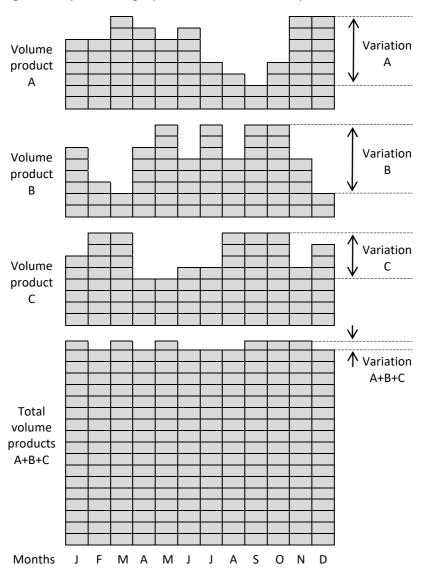
Let's look at the diagramme from the previous page. Here are three products: A, B, and C. As construction and technology, they are similar. Demand is different from month to month. We are able to produce equally efficiently, regardless of the length of the monthly series. If we take into account the different demand and put them on the same production line, we have a levelled production flow.
