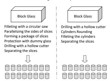
If we compare the two different technological sequences, shown at the previous page, it turns out that there is a difference in the number of operations. In the right-hand technological scheme, some operations are superfluous and avoided. We have reduced the number of operations from six to only four operations. This shortens the total lead time and reduces the number of sources of errors.
