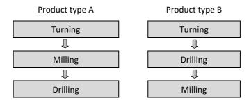
In the scheme above we look an example of mechanic operations. For product type A, the technological sequence is turning, milling, and drilling. For product type B, the technology starts from turning, but drilling and milling haves switched places.
