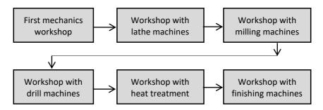
The scheme shows machine (workshop) organisation, in a factory for mechanic components. Given this type of organisation there are separate workshops, each specialised in the types of machines in them — a workshop for first machining, a workshop for lathe machines, a workshop for milling machines, a workshop for drilling machines, a workshop for heat treatment, and a workshop for finishing.
