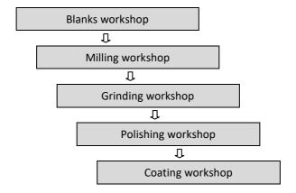
On the diagramme of previous page, we can see five production workshops. The process runs in the order of workshops. Various operations are carried out in each of them – preforming, milling, grinding, polishing, and applying optical coatings.
