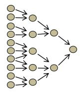
Inverse Tree-Like Flow is typical of assembly industries. There is a multistage flow of processing and manufacturing operations, as well as interim and final assemblies. A wide variety of materials, parts, elements, and components go into the production of systems and aggregates before reaching one or a range of final products. In an ideal case, all the times of the operations should be synchronised across all multistage flows. A pipe dream that we can't make happen...
