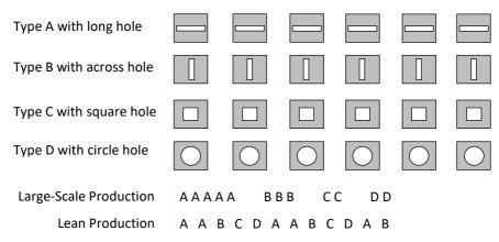
Now I will show how to achieve flow levelling "by nomenclature". Here are four types of metal plates – A, B, C, and D. Type A has a horizontal hole. Type B has a vertical hole. Type C has a square hole. Type D has a round hole. In a large-scale production, we first produce the entirety of plates type A, then the entirety of type B plates, then the entirety of type C plates.
