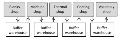
A water pump factory makes four families of pumps. Technologically organised sequential production flow: blanks shop, machine shop, thermal shop, coating shop, and assembly shop. There are buffer warehouses between the workshops.
