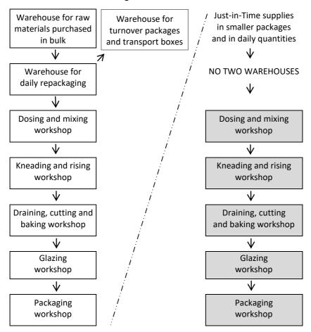
Here we are at another dry pastry factory. The production takes place through five separate workshops – a dosing and mixing workshop, a kneading and rising workshop, a pastry rolling, cutting, and firing workshop, a glazing workshop, and a packaging workshop. We see three warehouses before production workshops.
