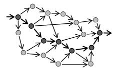
Network flow is typical for shipbuilding, construction, heavy machinery building industry, and other project-organised sectors. The so-called Critical Path is of key importance. The Critical Path is that continuous sequence of operations in which all the operations are without reserves of time and/or work resources.
