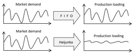
And so we get to Heijunka. On the left top and bottom of the chart is market demand, i.e., customer orders. They enter production in the form of production orders. If the sequence of production orders follows the sequence of customer orders (FIFO: first accepted, first introduced), like the customer orders flow varies, in the same way, the production flow will be subjected to widely variations.
