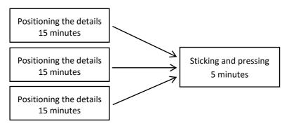
When, through Kaizens and whatever else, we expand the capacities of the main operations, we do not think to expand the capacities of the auxiliary operations.
