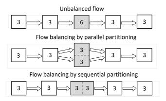
An unbalanced production flow with unequal operation times is seen on top of the scheme. The time of the first operation is three minutes; of the second operation is too three minutes; but of the third operation is six minutes, not three minutes.
