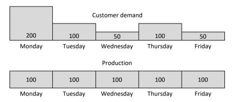
What is shown in the previous picture is now depicted in the form of bar charts. It is clear how the uneven demand (from 200 to 50 units per day, see above) has been transformed into levelled production (100 units every day, see below).
